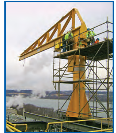
A Spanco Two-Ton 100-Series Freestanding Jib Crane with a 50-foot span trussed boom. The crane is mounted to the existing structure of a coal plant on the Susquehanna River. It is used to replace large coils that are part of a steam duct system.
