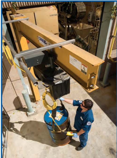
A water treatment plant uses this Spanco Two-Ton 200-Series Full-Cantilever Mast-Style Jib Crane at its receiving dock.
