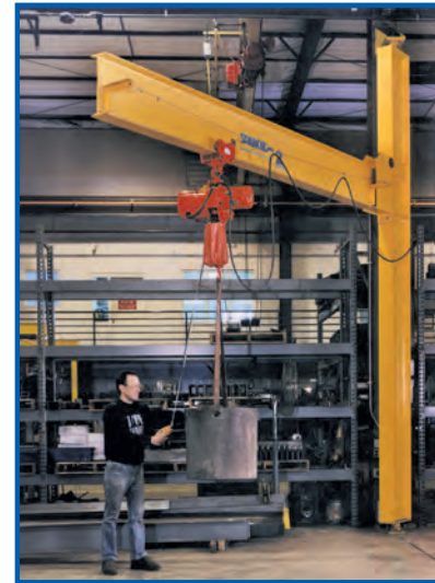
Spanco 201-Series Mast-Style Drop-Cantilever Jib Cranes are similar to the 200-Series Full-Cantilever Jib Cranes, with the addition of side-plate connections to "drop mount" the boom permanently at a specified height on the mast. This design allows for clearance from overhead obstructions located below the top of the mast.
