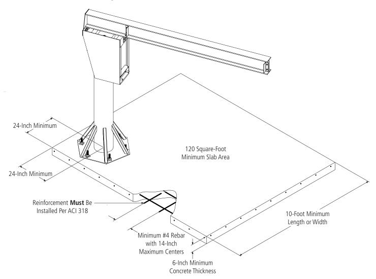
**NOTE:** The illustration above shows a 600 Series Jib. Foundationless jibs can also be 605 Series Jibs.
