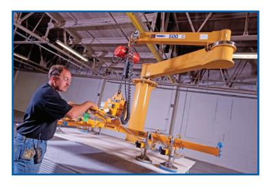
This Spanco 500-Pound Freestanding Articulating Jib Crane includes a customengineered, inverted knuckle boom to provide additional headroom.
