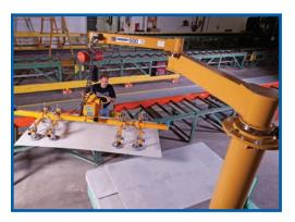
A Spanco 500-Pound Freestanding Articulating Jib Crane with an inverted outer arm and vacuum attachment for easy lifting
