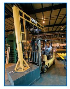
Freestanding Workstation Jib Crane with Portable Base
