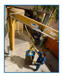
Spanco 200-Series Mast-Style Full-Cantilever Jib Cranes: the cantilevered boom is mounted at the top of the crane's mast to provide maximum clearance beneath it.
