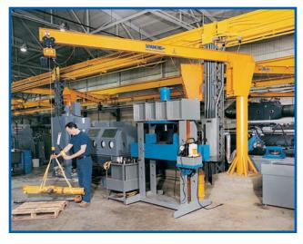
A One-Ton Spanco Freestanding Jib Crane used for shipping and assembly.
