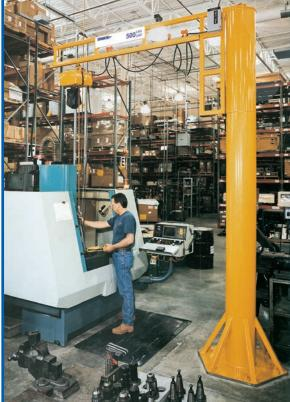
Parts are carefully lifted and positioned into this machine tool using a Spanco 500-Series Freestanding Workstation Jlb Crane.
