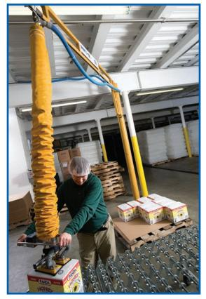
A worker stacks boxes of packaged food onto a pallet using a Spanco 150-Pound Capacity Freestanding Workstation Jib Crane with a vacuum attachment.
