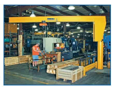
A Spanco 102-Series Freestanding Jib Crane lifting solid metal bars weighing up to 1/2 ton.
