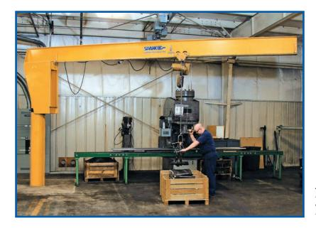
A worker lifts parts into a metalworking machine using a Spanco ½-Ton 101-Series Freestanding Jib Crane.
