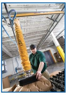
Like all Spanco Bridge Cranes, this ceiling-mounted system is compatible with numerous hoists, manipulators, and balancers. In this plant, a vacuum lifter is used to palletize large sacks of flour.
