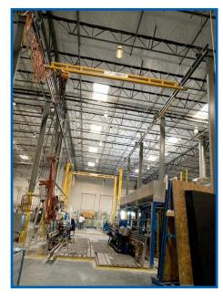
A custom-engineered 2,000-pound capacity Spanco Freestanding Bridge Crane designed for a glass manufacturer.
