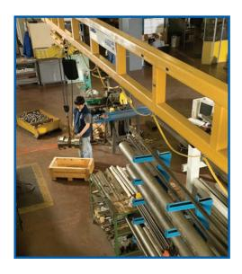
A coupling manufacturer installed several 4,000-pound capacity Spanco Freestanding Bridge Cranes to allow workers to move heavy loads from one work area to another with precision and accuracy.
