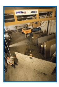
Storage and retrieval of granite countertops is a one-man task using this 2,000-pound capacity Spanco Freestanding Bridge Crane.
