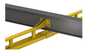
**Save Headroom:** A unique option to save headroom is to mount the header beam through the truss of the runway track, if the inside of the truss is tall enough to fit the header. For example, for four-column systems, you can mount the top tube of the runway track to the top of the header and sit the truss between the columns.
