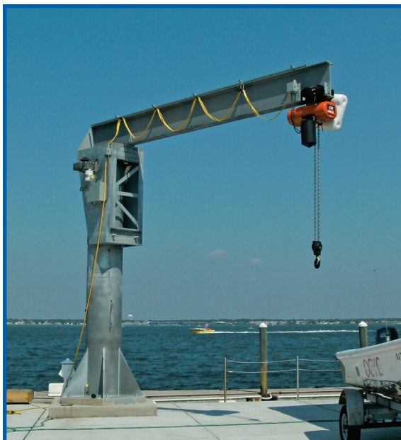
A large Spanco 100-Series Freestanding Jib Crane that's been galvanized to protect against sea spray and a corrosive outdoor environment. The jib was installed to lift boats easily at a protected, still-water marina.
