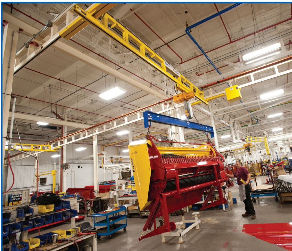
An agricultural equipment manufacturing operation using a freestanding workstation bridge crane with runways supported by steel columns.
