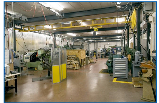
An example of the enormous coverage area possible with Spanco Bridge Cranes. In this case, one freestanding system provides overhead lifting for virtually every workstation in the shop.
