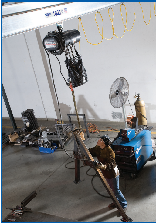
A worker uses a 1,000-pound capacity Spanco Alu-Track Bridge Crane to position product in her work area.
